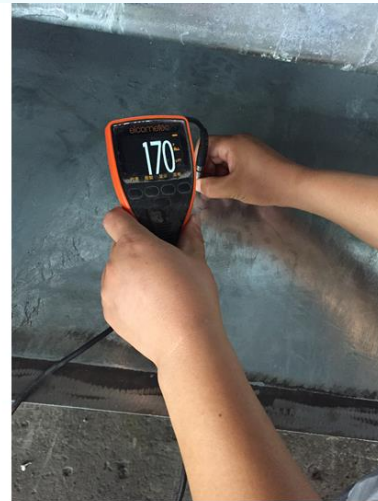
Checking of Thickness of Galvanizing Layer
